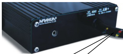
External connection cable and power cable
